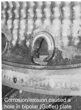
Fig 4 Perforated goffer plate
